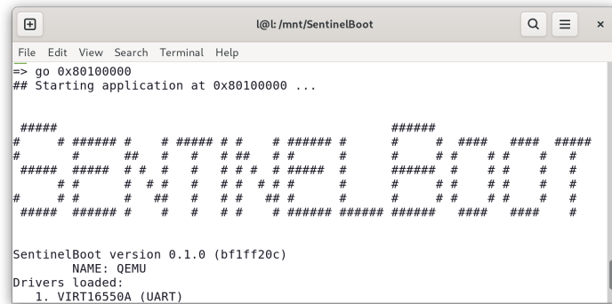
Figure 3.18: UART output in QEMU
